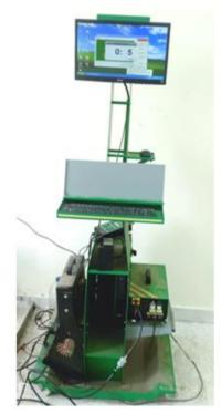
Fig. 5: Photograph of computerized gas analyzer
