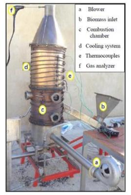
Fig. 3: Photograph of the biomass boiler in operating mode.
