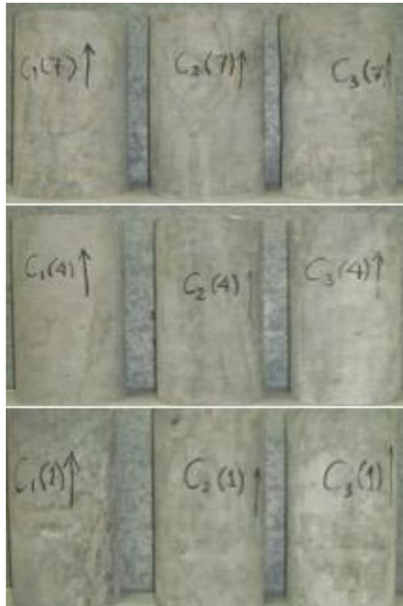
Fig. 9 The final stage of cylinders cut showing the surfaces from the three columns cast. These pictures evidence non-porous cylinder columns.
