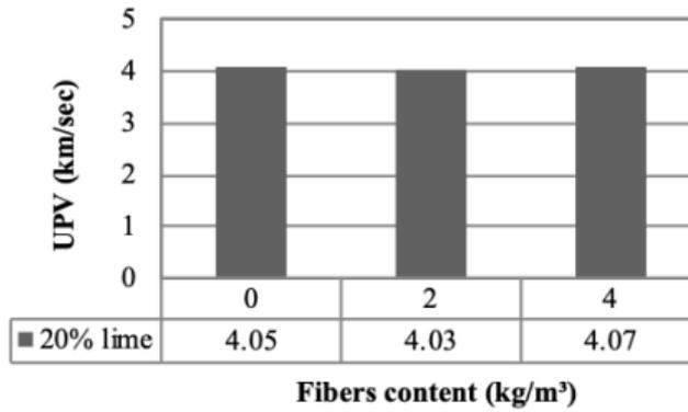
Fig. 8 UPV vs linen fiber content.
