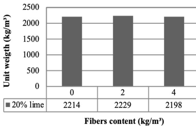
Fig. 6 Unit weight vs linen fiber content.
