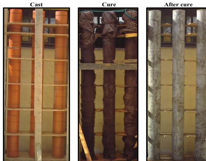
Fig. 1 Slender Column of specimens for (casting, curing, & after curing).
