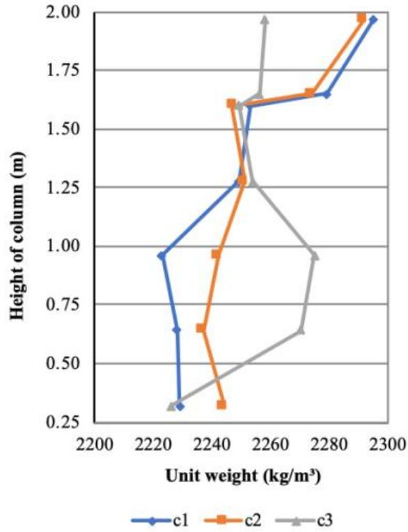
Fig. 10 Variation of unit weight along the columns.
