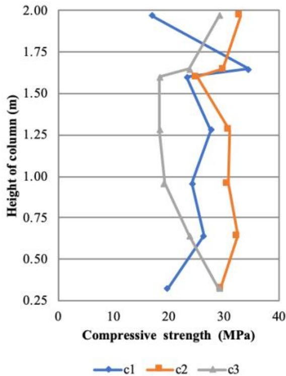
Fig. 11 Variation of compressive strength along the columns.
