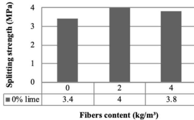
Fig. 5 Splitting strength vs linen fiber content.
