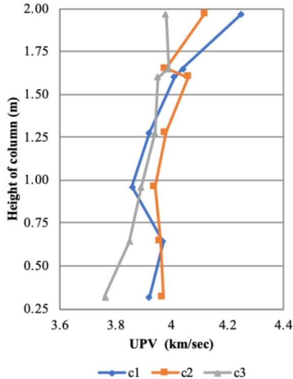
Fig. 12 Variation of UPV along the columns.
