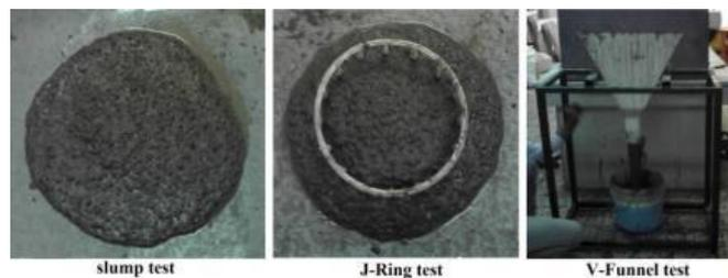
Fig. 3 Test specimen of SSC; “Slump test, J-Ring test, & V-Funnel test”.
