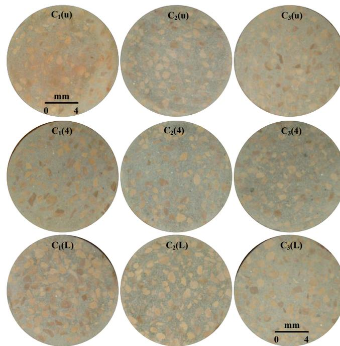
Fig. 13 Distribution of coarse aggregate along the column's height.
