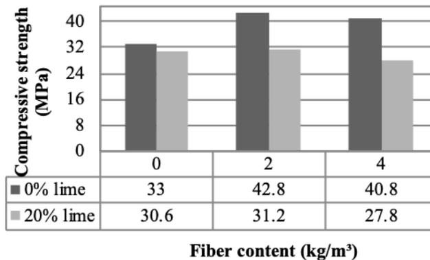
Fig. 4 Compressive strength vs linen fiber content.
