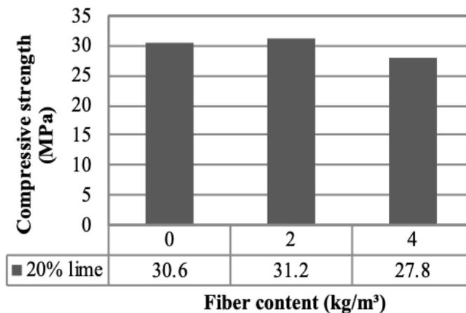
Fig. 7 Compressive strength vs linen fiber content.
