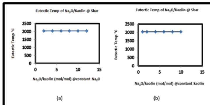
Figure 3 4: (a) Eutectic temperature between kaolin and Sodium oxide at constant Na<sub>2</sub>O, on binary phase diagram at 2000 °C. (b) Eutectic temperature between kaolin and Sodium oxide at constant kaolin, on binary phase diagram at 2000 °C
