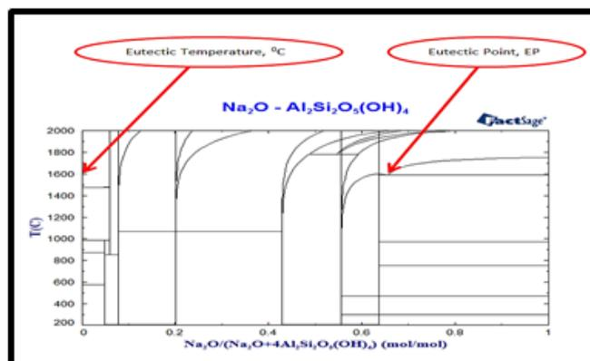
Figure 4.1: Profile of eutectic points on binary phase diagrams at  $1600^\circ\text{C}$
