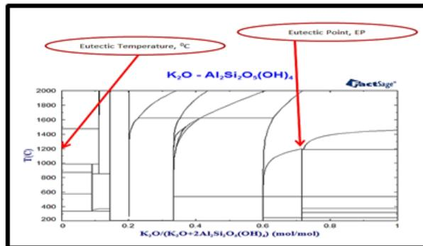
Figure 3-3: Profile of Eutectic points on binary phase diagrams at 1200 °C
