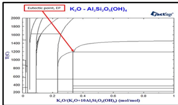
Figure 3-1: Profile of Eutectic points on binary phase diagrams at 1200 °C
