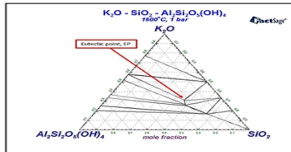
Figure 4-2 Profile of Eutectic point on a ternary phase diagram at  $1600^\circ C$ , 1 bar
