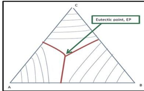
Figure 2-2: Schematic of Eutectic point on a typical ternary phase diagram [5]
