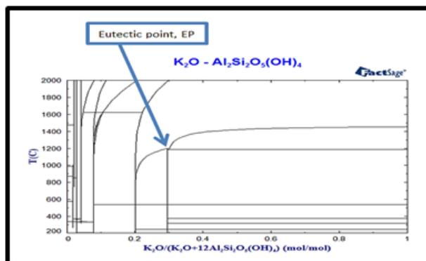
Figure 3-2: Profile of Eutectic points on binary phase diagrams at 1200 °C
