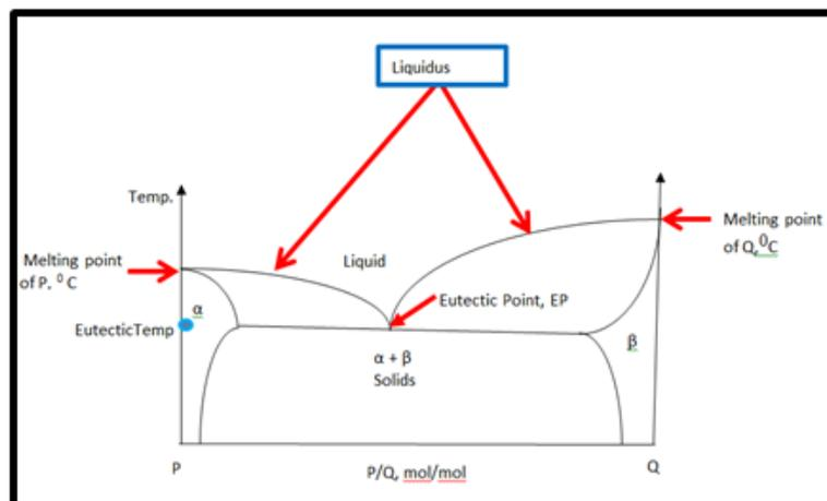
Figure 2-1 Schematic of a eutectic point on a typical binary phase diagram [5]
