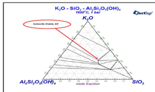
Figure 4-3: Eutectic point at  $1650^\circ C$ , 1bar on ternary phase diagram
