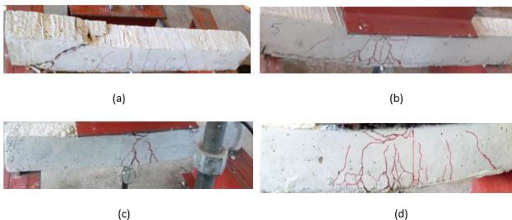
Fig. 4. Failure Mode of Beam Samples: (a) Sample Type-A3, (b) Sample Type-A5, (c) Sample Type-A1, and (d) Type-A4
