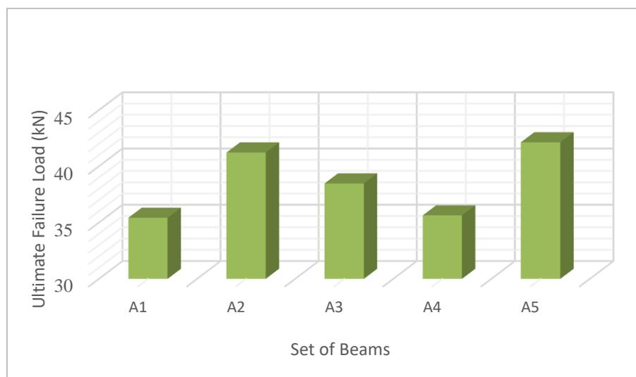
Fig. 3: Ultimate failure load (kN) of Sample Type
