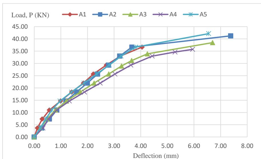
Fig. 2: load against deflection at mid-span
