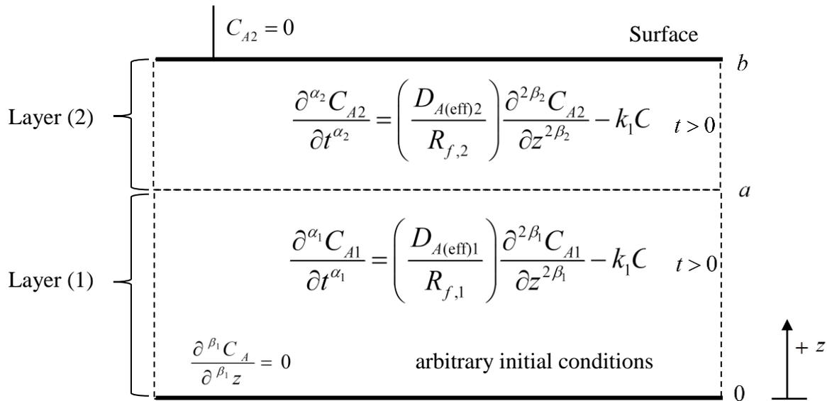
If we write equations (1) and (2) in fractional differential equations [2] we have :
