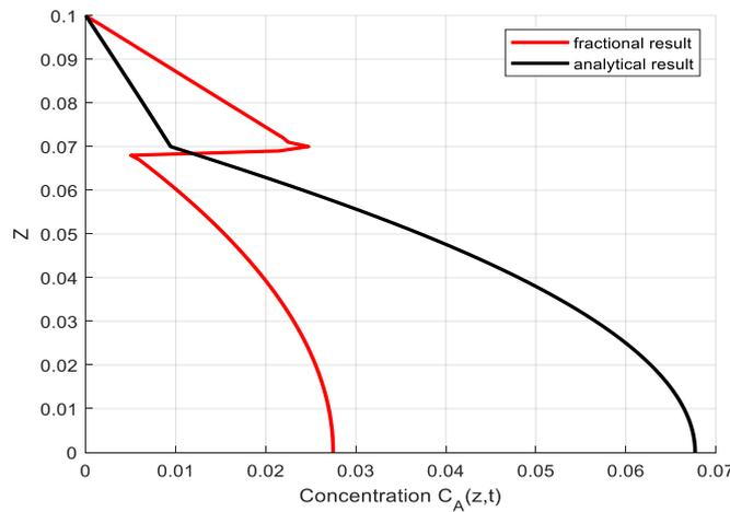
Figure 7 : Comparison of analytical and fractional methods for  $0.59 = \alpha_1 \neq \alpha_2 = 0.61$
