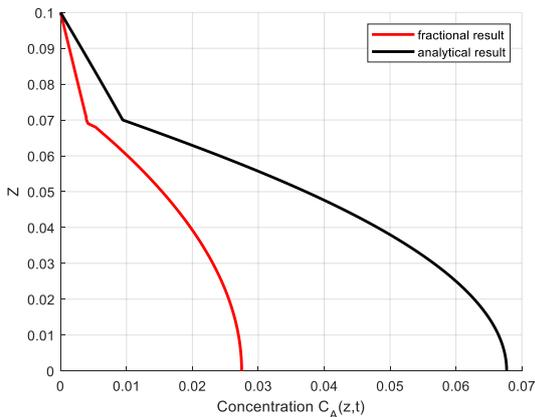
Figure 5-c : Comparison of analytical and fractional methods  $\alpha_1 = \alpha_2 < 0.6$
