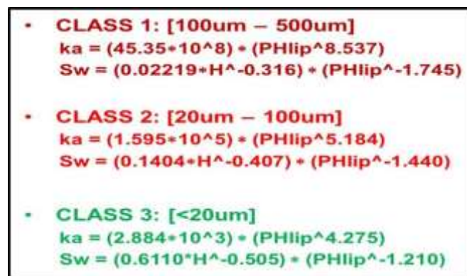
Figure 4 : Equations for Calculating Sw and ka from Lucia (1995)
